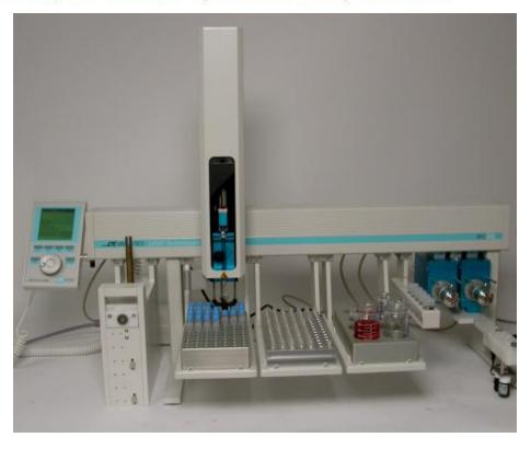
The PAL offers precise control of the down force on the sample. The user can specify the speed of compression in the method, allowing even very heavy suspensions to be filtered successfully.
