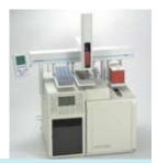
Static Headspace - Liquid Injection - SPME - ITEX Extraction combined in one single instrument
