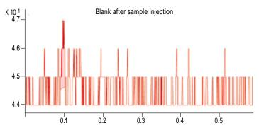
Injection of 272 .2 pg Dextromethorphan on column; followed by blank injection No carryover could be detected.
