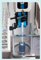
Semi-Solids require a disposable positive displacement tip and an analytical balance in order to meter exact quantities into an empty vial.
