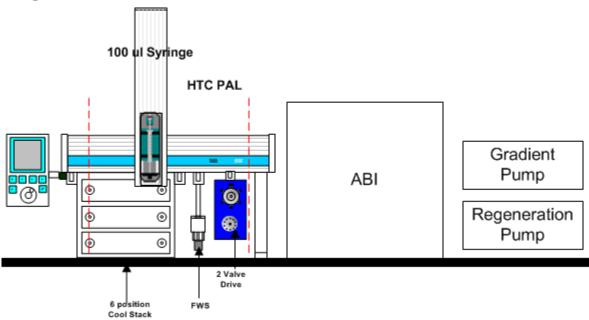
**LEAP System** consists of an HTC or HTS PAL with (1) 6 port valve and drive for injection, (1) 10 port valve and drive for column selection, (1) LEAP Standard Cycle to be used in Analyst, ICC-CE software, (1) Fast Wash Station, (1) cable, and installation & training.
