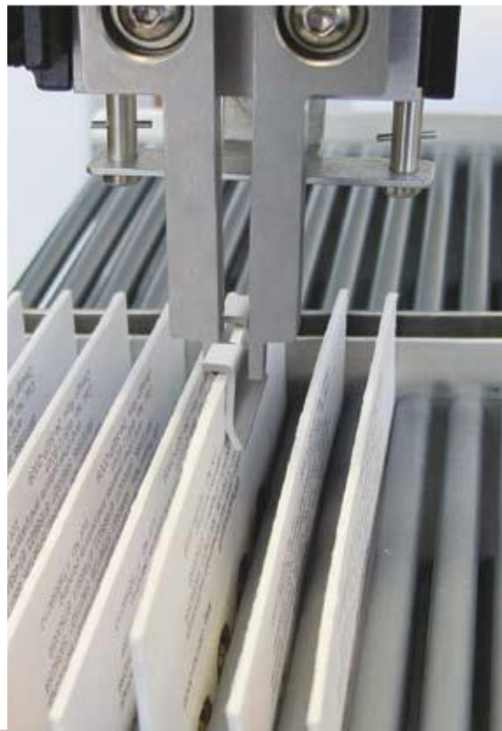
SCAP DBS system robotic gripper tool picks up DBS card ... ..and places it into the DBS SCAP system clamp module where the DBS card is implemented into the analytical flow
