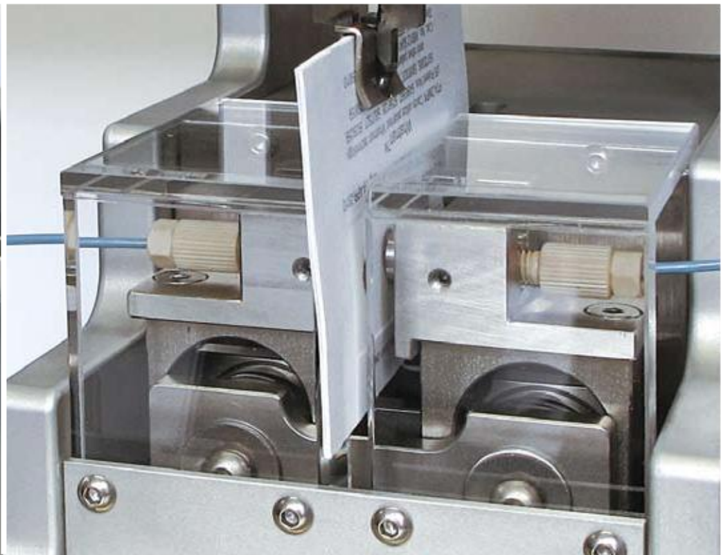
SCAP DBS system robotic gripper tool picks up DBS card ... ..and places it into the DBS SCAP system clamp module where the DBS card is implemented into the analytical flow
