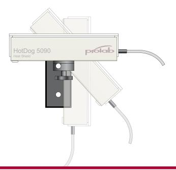
The Hotfix 5090 serves as the Hotdog 5090's holder for the CTC PAL autosampler and can be mounted close to the injection port to reduce the length of connection / transfer lines.
